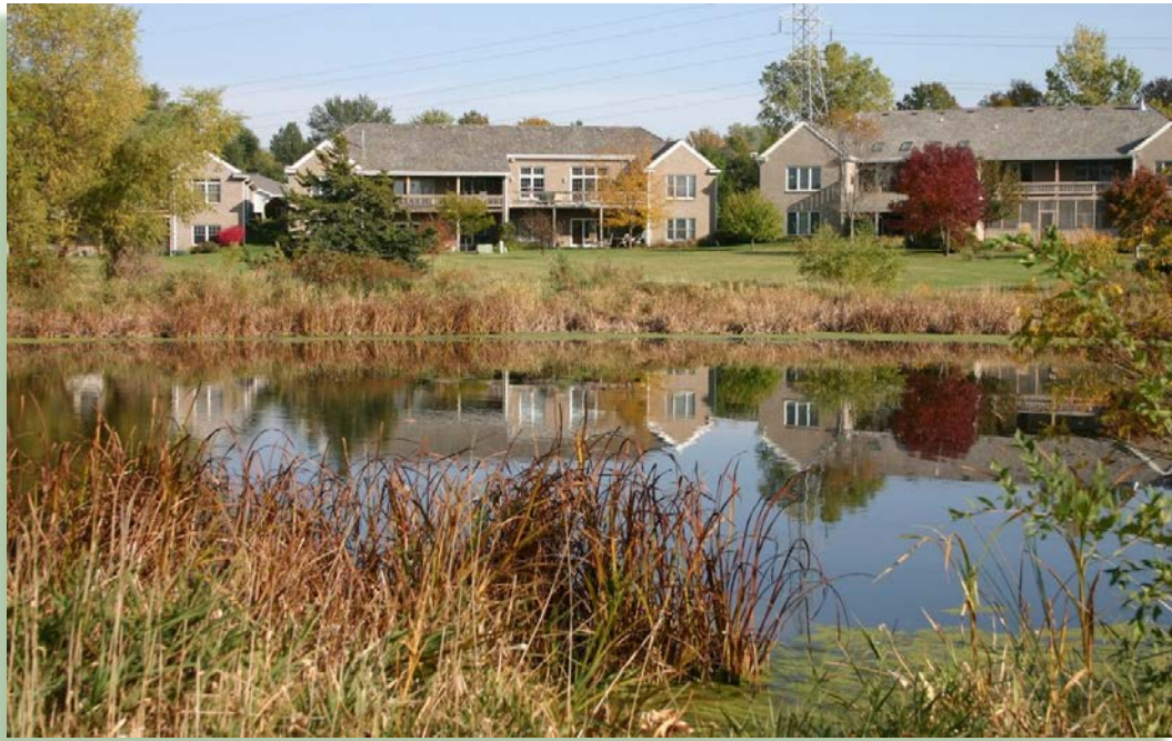
Detention ponds should be a landscape feature with a natural shape, not a geometric shape.
